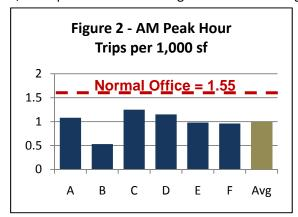
period between 7:00 and 9:00 a.m.). The highest rate observed in the morning rush hour was 1.25 trips per 1,000 square feet while the lowest was 0.53 trips per 1,000 square feet. The average trip rate was 0.99 trips per 1,000 square feet, which is a 36% reduction in trips compared to the industry average rate of 1.55 documented in the Institute of Transportation Engineers' *Trip Generation*, 8<sup>th</sup> Edition. All six sites have a rate lower than industry average.
